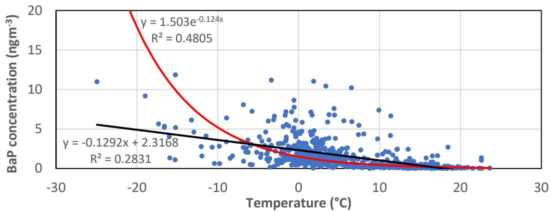
**Figure 1.** Daily average concentrations of benzo(a)pyrene versus air temperature. Fitted linear trendline is shown in black and exponential trendline in red.
